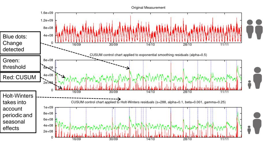
From Gerhard Münz. Traffic Anomaly Detection and Cause Identification Using Flow-Level Measurements. PhD thesis, Technische Universität München, June 2010. Anomaly Detection (2)
