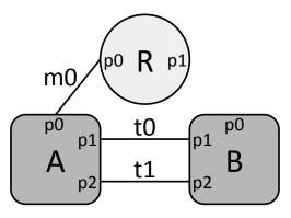
Figure 2: Example topology consisting of the management router R and testbeds A, B
