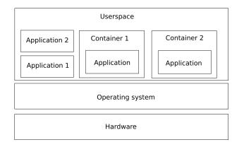
Figure 2: Scheme of container-based virtualization. Hardware and Kernel of the host are used, containers are running in userspace separated from each other.
