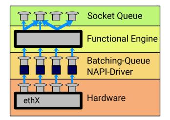
Figure 1: Inner Structure of PFQ, Image was redrawn and adapted, original by Bonelli et al. [2]
