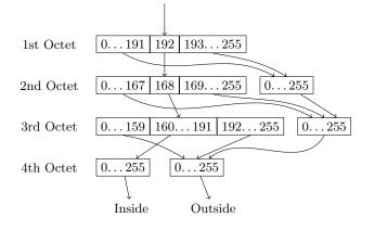
Figure 3: Example of how ITVal [19] would represent a match for 192.168.160.0/19, given that the packet consists only of a single IP address to match on.
