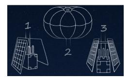
Figure 3: Main components of a balloon 1) solar panels 2) envelope 3) electronics[9]
