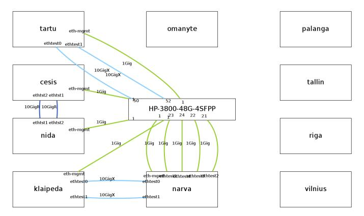
Figure 4: Generated partial topology map of the Baltikum testbed, 20.12.2015
